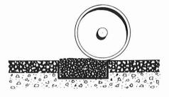
6. Compaction: It is crucial that the patch be compacted properly. Poor compaction will cause shrinkage of the patch, allowing intrusion of water around the edges and ultimately leading to failure.
