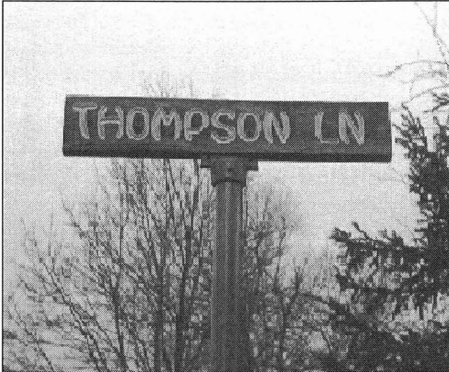
Signs like this one must be replaced in the near future with retroreflective signs.
