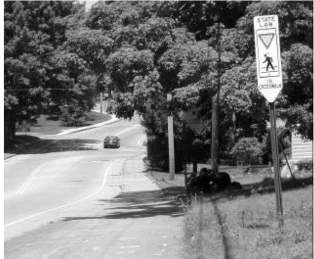
*Picture 3. The appropriate sign is a W11-2; not a Supplemental Crosswalk Identification Device*
