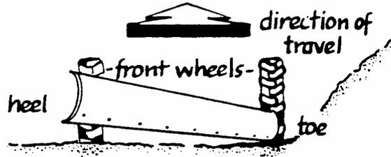
*Figure 2.1 Marker Pass Toe tight & heel raised. . .*
