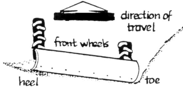
*Figure 2. 2 . . . set the blade tight on both ends*
