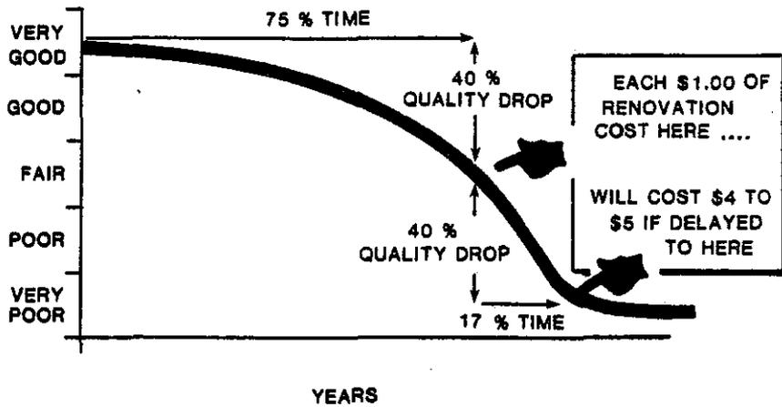
Above: As the years increase, the PCI rating (measurement of the structural integrity and surface condition of a road) decreases dramatically and the cost of maintenance/rehabilitation increases.
