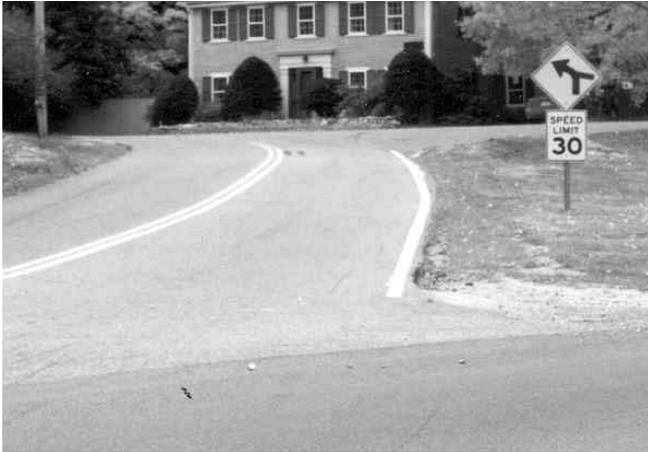
Figure 1. An improperly installed Speed Limit Sign (R2-1)
