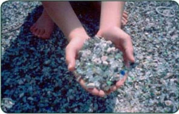
*Pulverized recycled glass after processing ready to be used in roadway projects.*
