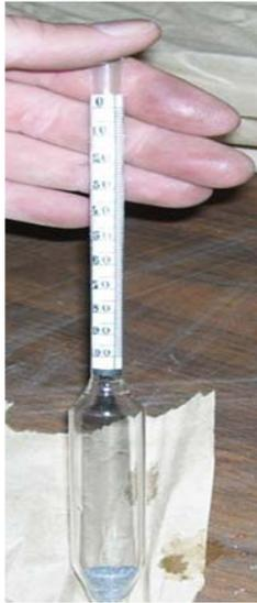
*The hydrometer measures the level of the salt brine.*
