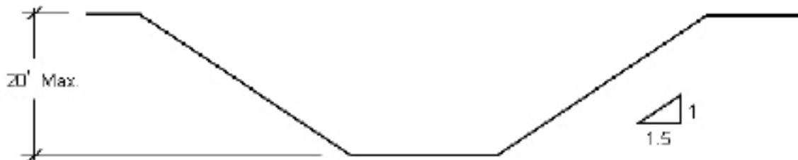
Figure 2: Culvert trench side slope (OSHA)
