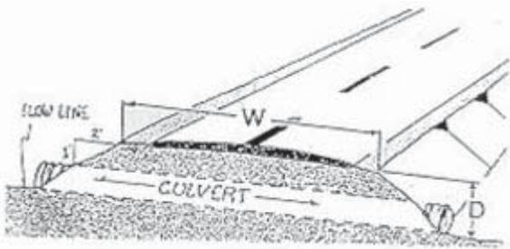
Figure 1 – Road cross-section showing culvert slope (Skorseth, Place Culverts Correctly the First Time)
