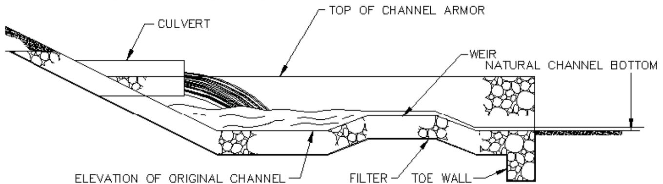
Figure 7: Weir-formed Plunge Basin
