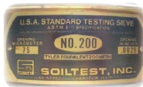
*Top: A USA Standard Testing Sieve No. 200.*
