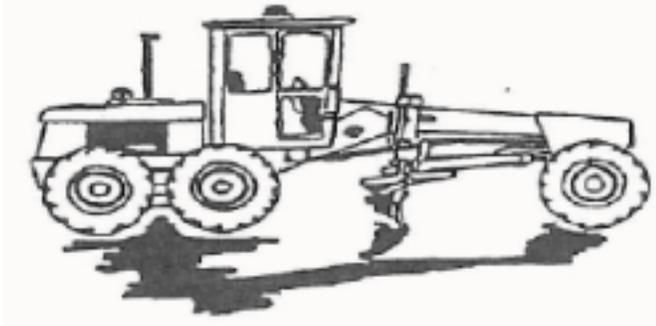
Reshape the roadway, shoulders, and ditches regularly. Maintain about a 4% (or 1/2 inch per foot) crown on the roadway with as little deviation as possible. Use a grader to create a crown that follows a straight line from the centerline of the road to the shoulder.
