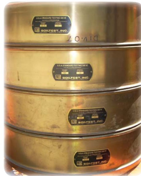
On Left: A USA Standard Testing Sieve. The opening in millimeters and in inches is listed on each sieve.
