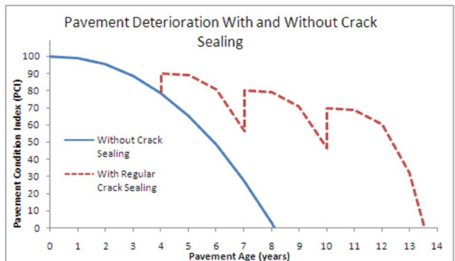
Figure 2: Pavement Deterioration With and Without Crack Sealing
