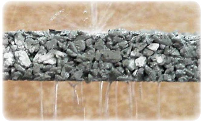
Figure 1: A typical cross-section of a pervious pavement.
