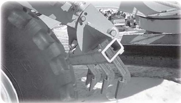
*Figure 1: A grader-mounted scarifier is generally a poor tool for breaking snowpack due to great potential for road surface damage.*
