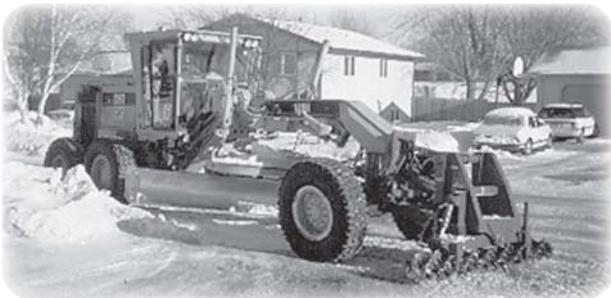
*Figure 2: An IceBuster mounted on a grader.*
