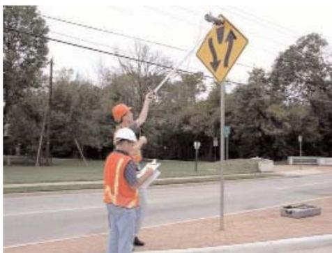
Retroreflectometers are used to measure sign retroreflectivity.
